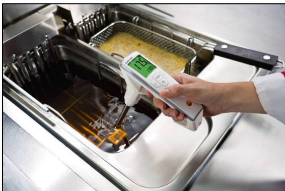
Figure 1: TPM Meter Used to Monitor Oil Quality. The simple operation of the meter allows anyone to test oil quality. The only condition for the meter is a minimum of five minutes should elapse after fryer use before recording a reading because actively frying food will interfere with the measurement. Image from www.testo.com
