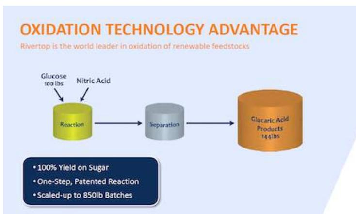
Figure 14. Rivertop Renewables Process to Glucaric Acid.
