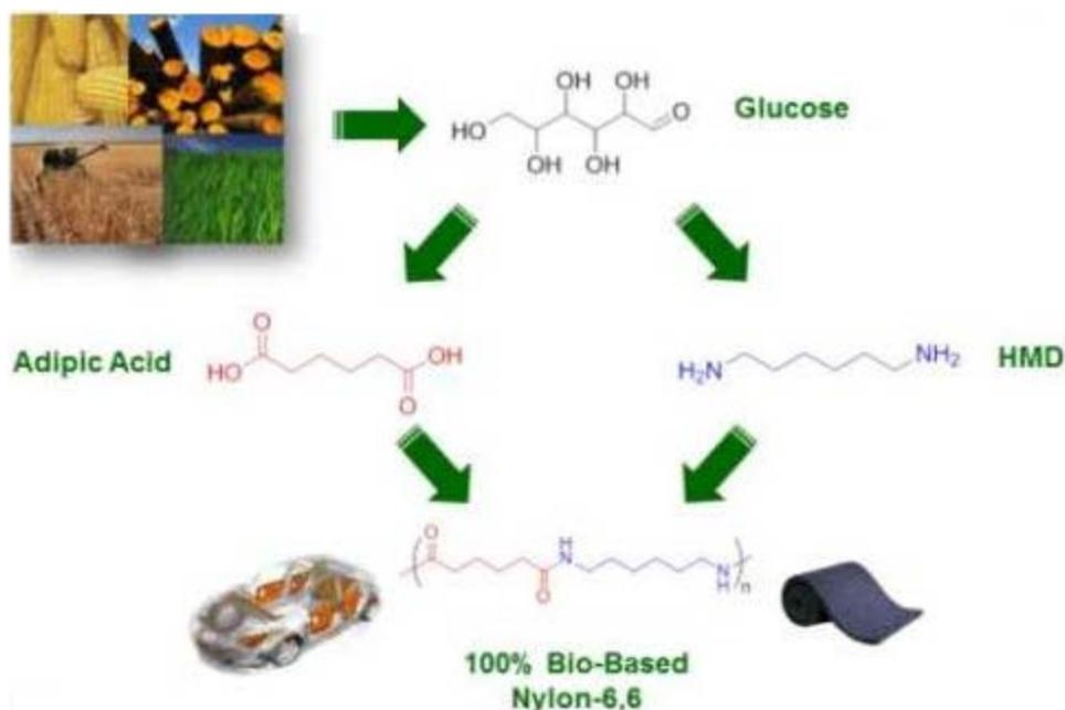
**Figure 13. Rennovia Process for Hexamethylene Diamine.**
