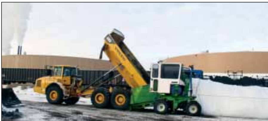
American Crystal Sugar in East Grand Forks bagged more than 3,000 tons of beet tailings and pulp left over from the sugar-making process. Converting the tailings into silage preserves the nutritional value, plus reduces the expense of land applying waste tailings by making the silage available to local livestock producers.
