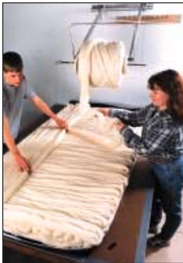
High Pointe Coverings employees arrange seven layers of 4 to 5 inch-thick pure, carded wool, using 34 to 35 pounds of wool per mattress.
