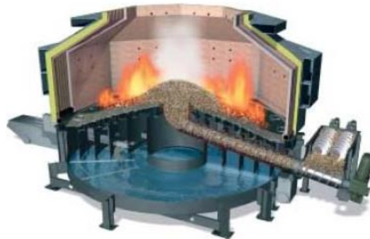
Figure 4. Central Lower Biomass Feed System
